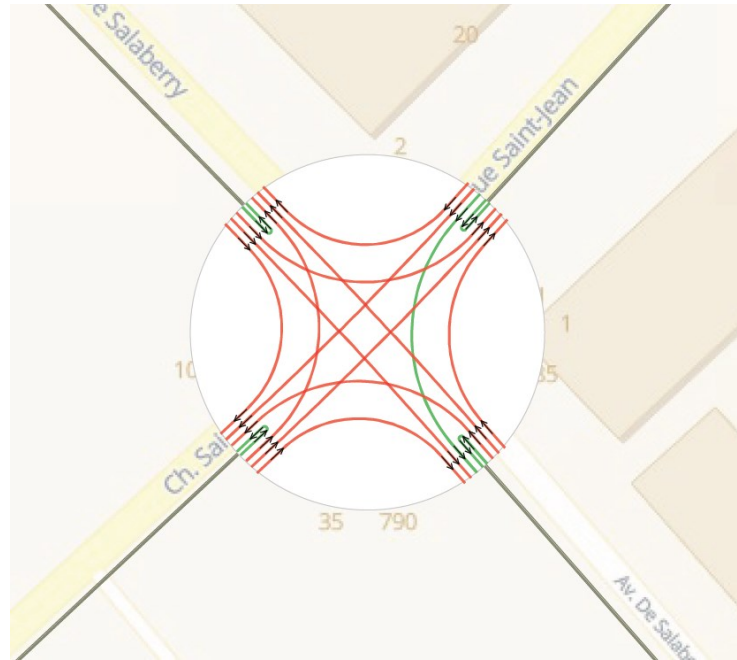
Figure 3-9. Extracted intersection movement permissions
