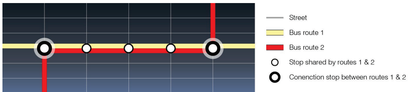
Figure 13: Connection stops between overlapping routes
