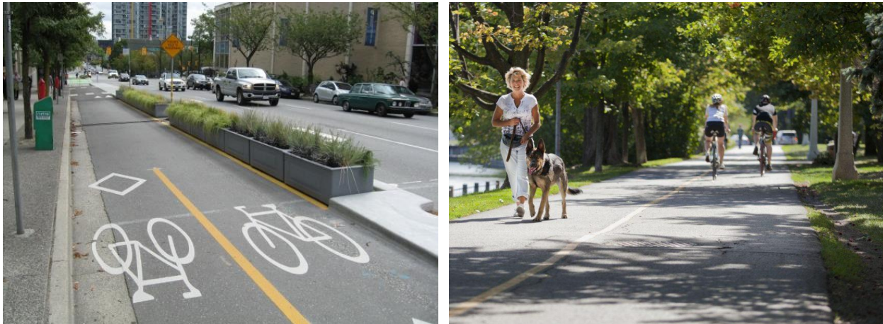
Figure 6. Cycle track (left) and bike path (right). Sources: Livable Cities (left) and NCC (right)
